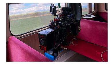
Luckily, using Ncam's Mk2, the team was able to get as close as 50 cm to the markers, which were triangular reflective points Horký put on the ceiling of the train set. Using computer vision techniques to define a 3D point cloud representation of the surrounding environment, the Ncam software automatically determined the optimum tracking algorithm at any given point in time, leading to greater reliability and accuracy in the challenging environment.
